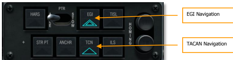
Figure 323. Navigation Mode Select Panel
