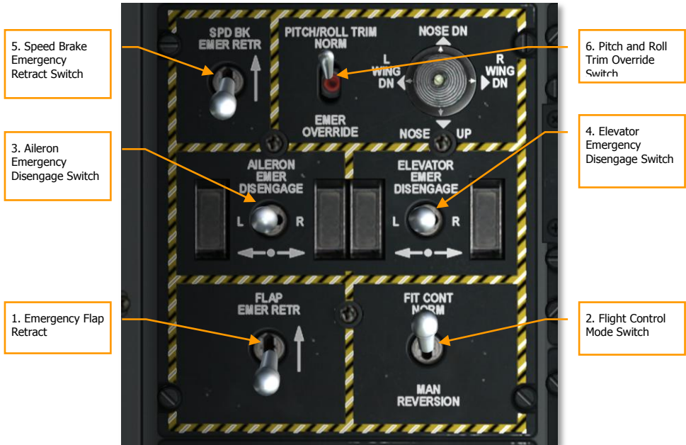
Figure 297. Emergency Flight Control Panel
