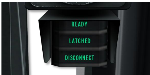
Figure 103. Air Refuel Status Lights
