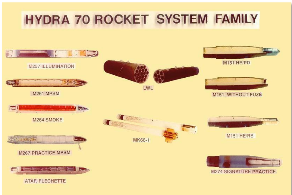
Figure 45. 2.75 inch FFAR Warhead Types
