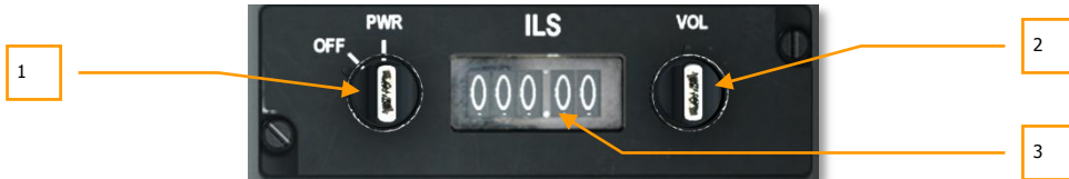
Figure 129. ILS Control Panel
