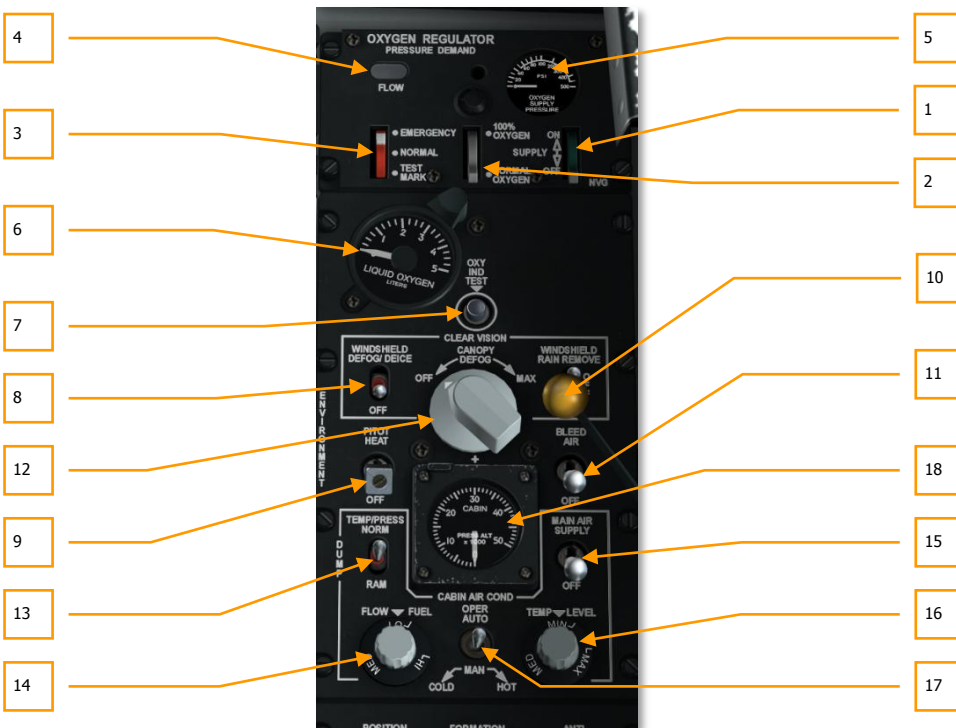
Figure 125. Environment System Panel
