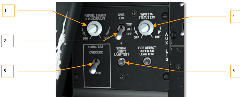
Figure 116. Auxiliary Lighting Control Panel
