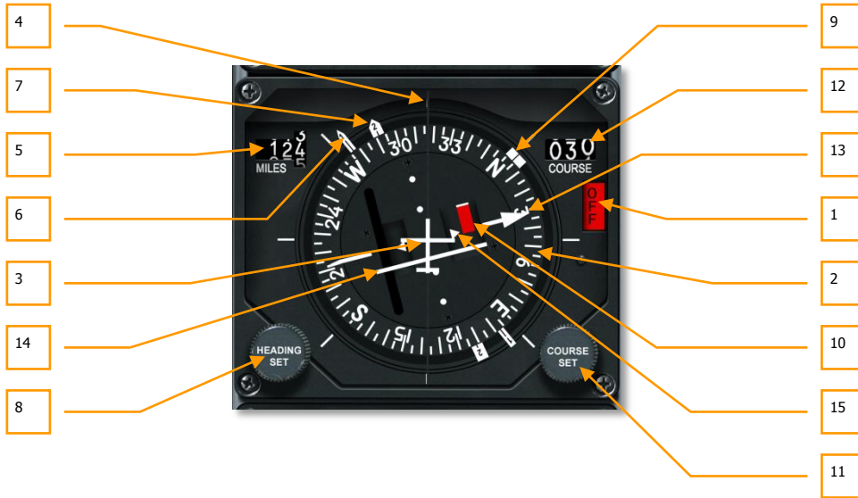
Figure 89. Horizontal Situation Indicator
