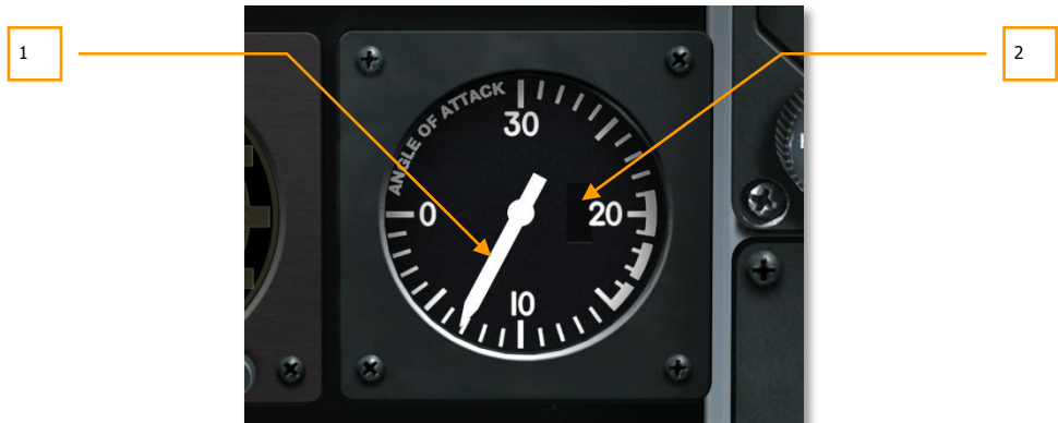
Figure 77. Angle of Attack Indicator
